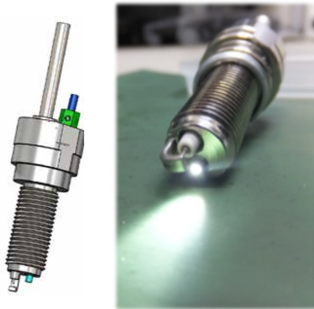
Fig. 2 Spark-plug sensor with optical fiber
