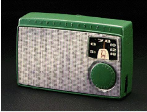
The first transistor radios could not receive FM because the frequency of around 100MHz was too high for the transistors of 1955 that could reach only 20MHz at best. To better the frequency range the transistor's
